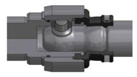
Cardan Joint: Cardan joint is the best solution for heavy application with high pressure inside the pump casing. It improves the allowable torque up to 4 times torque with the same pump size. It is available with internal metal joint protection to for an additional improvement of the rubber service life.
